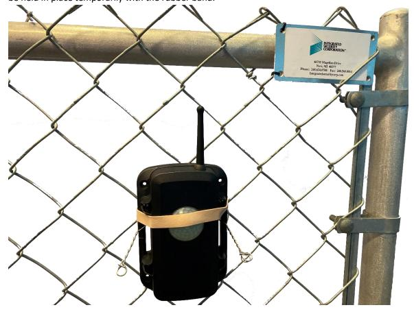
Using the Torque Limiter and provided screws, secure the cover to the case. Once all four screws are properly torqued, pull the zip ties tight to secure it to the fence.
