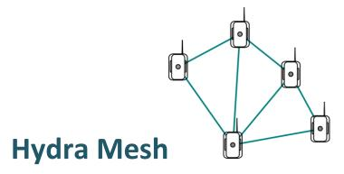
The Hydra Sensor Mesh network consists of a self-forming multi-hop, mesh of nodes which collect and relay data, and a network manager incorporated in the Hydra Gateway Board that monitors and manages network performance and security.
