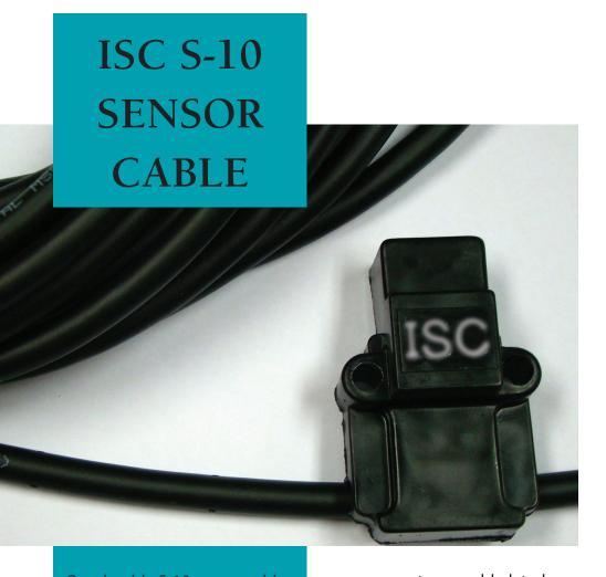
Our durable S-10 sensor cable is designed to give you years of maintenance-free service. The cable is direct burial rated and UV resistant. Inside, the zone wires give strength and abrasion resistance while the sensor is attached to a Teflon-coated inner connector. Shielding and a ground wire prevent electrical interference.
